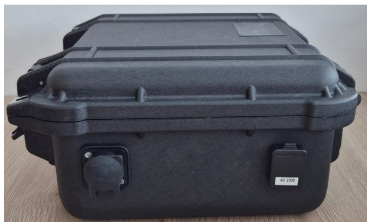
Figure 17: A view of the input solar panel and mains connectors on the charging case
