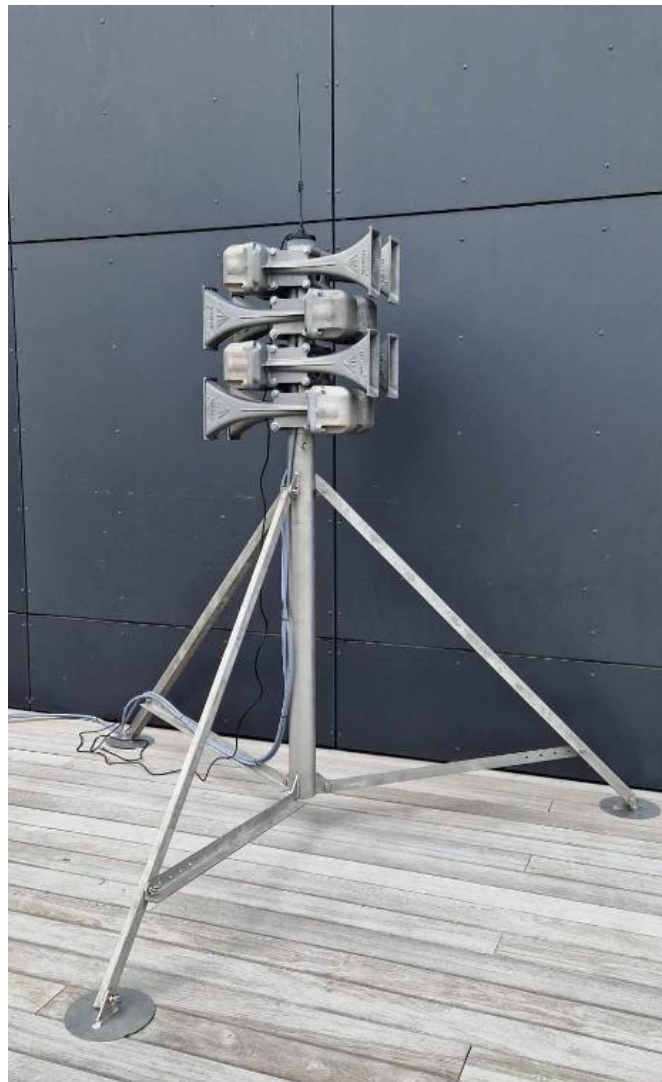
Figure 7: The 1,200 W loudspeaker assembly with an aerial on a standard tall tripod
