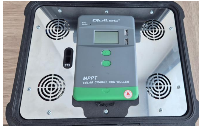
Figure 15: The solar-mains battery charger – an inside view of the charging case
