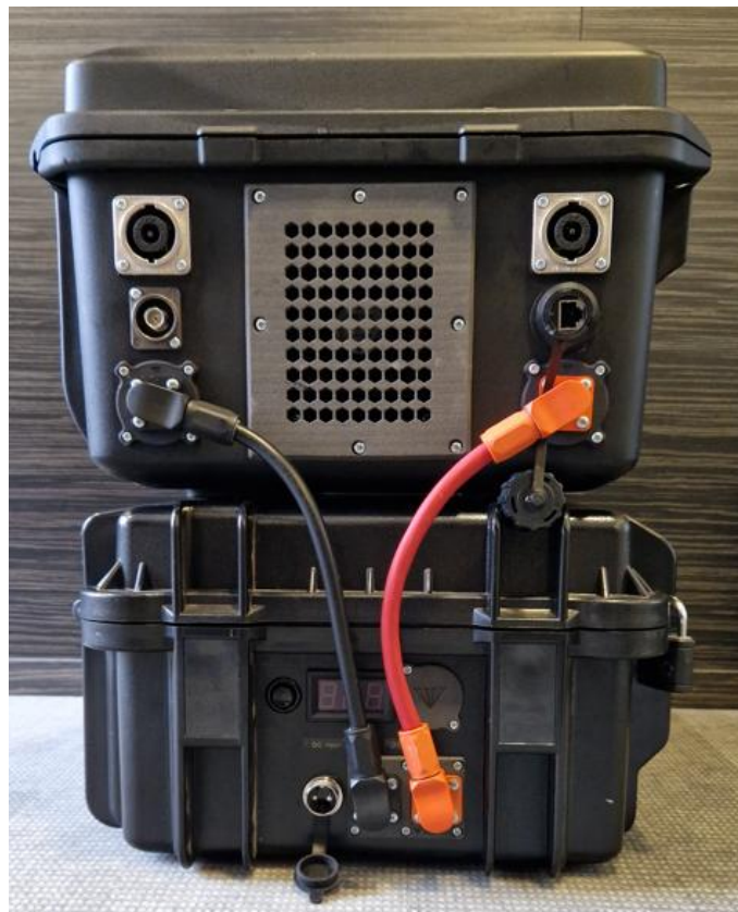
Figure 8: The power cables
